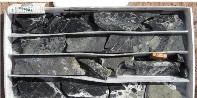
Photo of half-core from JM-DDH-14-10 Box 47 (104.70 to 106.95) before sampling quarter-core during 2015 verification program (Sample ID: 100060).
