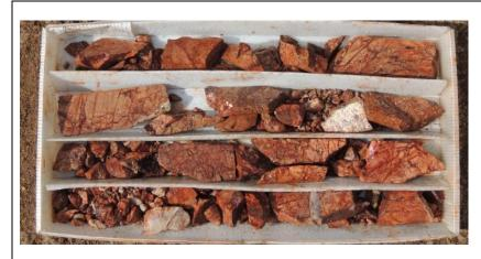
Photo of half-core from C-DDH-11-16 Box 23 (49.00 to 51.00) before sampling quarter-core during 2015 verification program (Sample ID: 100064).
