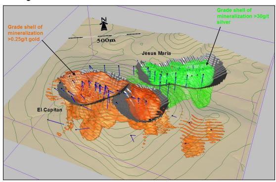
Figure 14-19: Isometric View of Grade Shells at Projected Cut-Off Grades Relative to Floating Cone Pit Shells
