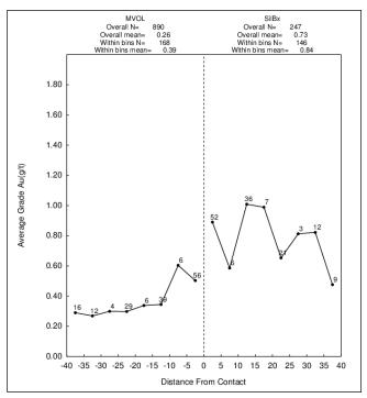
Figure 14-8: Contact Profile for Gold in Silicified Breccia Zone vs. Mineralized Sediments at El Capitan
