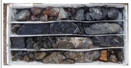
Photo of half-core from JM-DDH-14-10 Box 13 (27.70 to 29.75) before sampling quarter-core during 2015 verification program (Sample ID: 100059).
