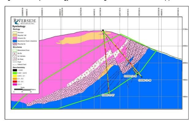
Figure 7-5: El Capitan Geology Section Showing Drill Holes and Structures (1)
