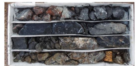
High grade silver vein mineralization at Jesus Maria – DDH-14-10: 2.1 m @ 1046 g/t Ag and 1.34 g/t Au
